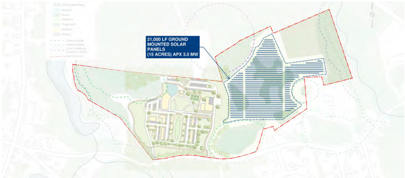
Fig 20. Potential Layout for Solar Panels
