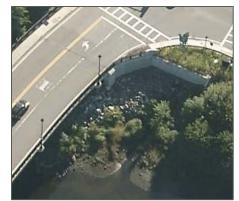
Scour at stormwater outfall to Merrimack River near Bates Bridge.
